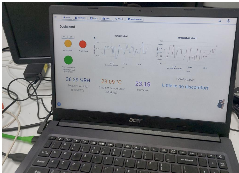
Figure C3: Development laptop acting as HMI, hosting FUXA, showing 'Dashboard' screen.
